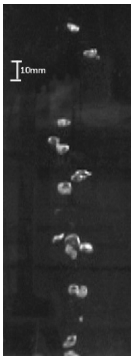
Fig. 1. Image obtained for interfacial area determination using the photographic method. [\text{DTABr}] = 10^{-5} \text{ mol L}^{-1} . Q_g = 24 \text{ L h}^{-1} .
